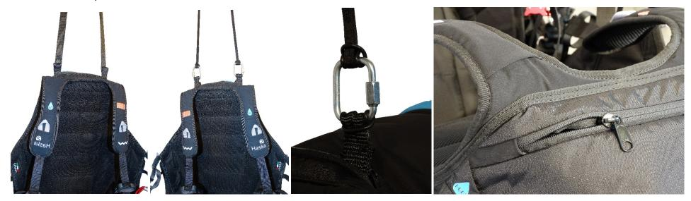
The two connections should be made using screw-lock karabiners with a breaking strength of at least 1,400 kg. In any case, it is important to verify that the length of the bridle is sufficient to position the reserve parachute inside the harness pocket, and that there is sufficient play to enable the parachute to be taken out of the pocket without causing the reserve parachute deployment bag itself to open during extraction.
